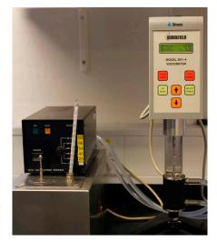
Figure 14: Equipment to test dynamic viscosity (cP)
