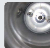
Varnish-like deposits were removed from metal surfaces.
