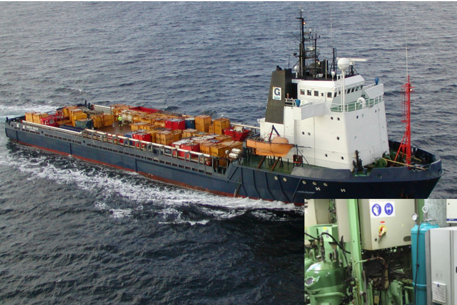
Supply Vessel Engines type BERGEN, 2,500 kW
