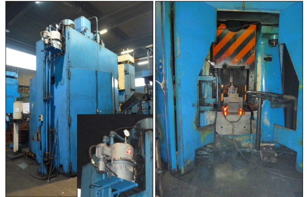
LASCO drop-forging hammer with CJC® Fine Filter unit 27/27
