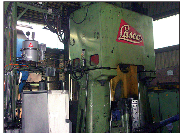
Lasco drop-forging hammer with CJC® Oil Care System 27/27
