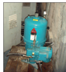
CJC® Oil-Care System installed at the hydraulic system of the vertical raw mill #4
