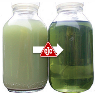
After the first filter pass Cleanliness class: 15/13/10 > 40 % less particles > 2 µm
