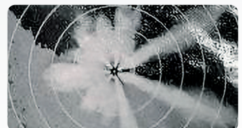
Changed spray pattern due to clogged and worn nozzles
