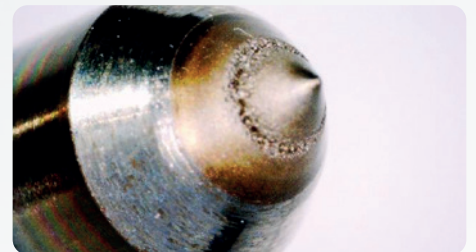
Cavitation and corrosion on injection nozzles
