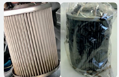
In-line oil filter Photos le: new filter, ri: quickly clogged filter
