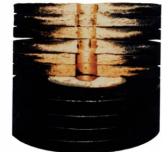
Cross-section of a used CJC™ Depth Filter insert
