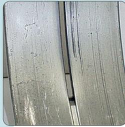
Grooving through abrasion (bearing ring)
