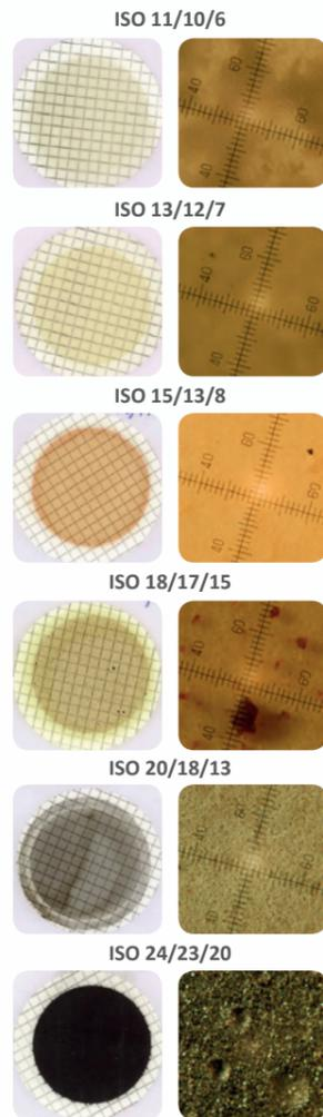
Photos of test membranes of various contamination degrees
