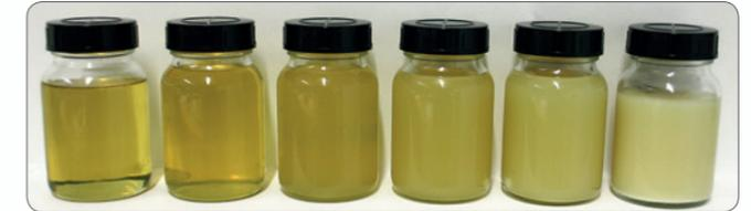
Hydraulic oil samples with various water content. From left: 0.01 % - 0.03 % - 0.06 % - 0.1 % - 0.2 % - 2 % water in oil
