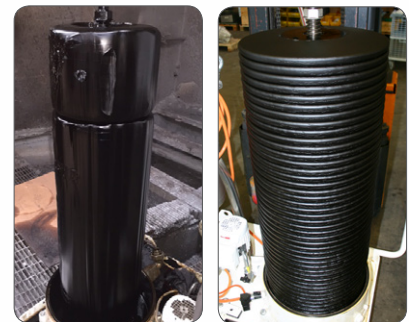
Filter insert replacement - clearly visible the extremely high dirt holding capacity
