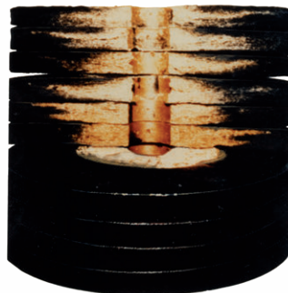
Cross-section of a used CJC™ Depth Filter insert
