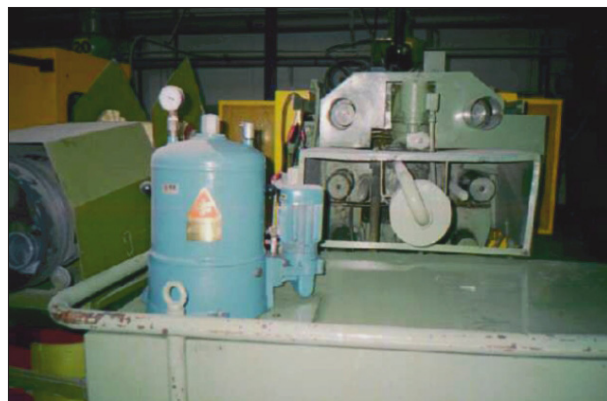
At Wavin Metalplast in Buk, Poland all STORK plastic injection moulding machines are equipped with CJC™ Fine Filter units.
